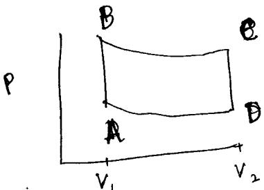
$$P_A V_1 = R T_A \quad P_B V_1 = R T_B; \quad P_C V_2 = R T_C$$
