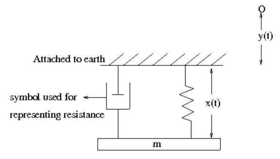
Let y(t) be the displacement of the platform with respect O, origin in an inertial frame. x(t) is the displacement of the mass m with respect to the platform. If  $y(t) = A\cos(\Omega t)$  show that
